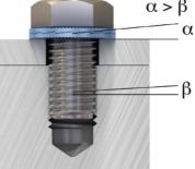
The Nord-Lock combi bolt secures bolted joints by using tension instead of friction. The cam angle ' $\alpha$ ' is greater than ' $\beta$ ', creating a wedge effect that prevents any unintentional loosening of the bolt.
