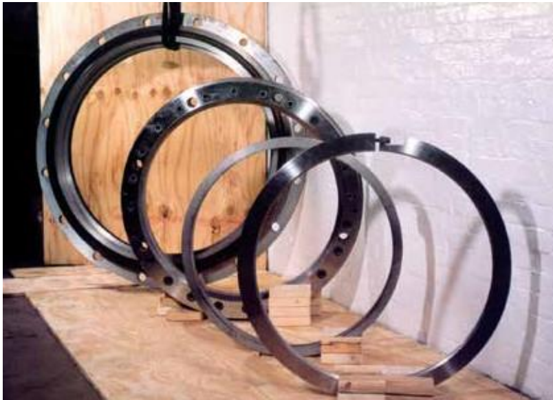
Example of Superbolt thrust collar: A modified thrust collar is retained in the chock, which requires only the manipulation of the split ring.
