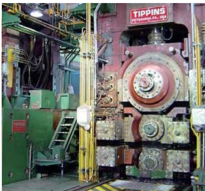
Multiple Superbolt Thrust Collars, as well as MT nut-style multi-jackbolt tensioners used on this hot strip mill.
