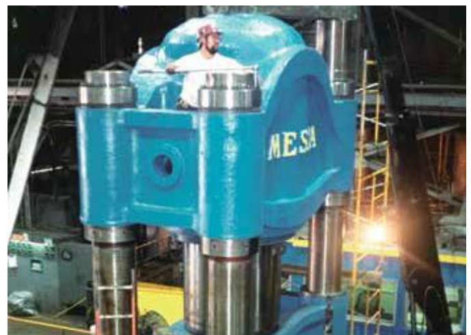
3,250 ton slab shear press.
