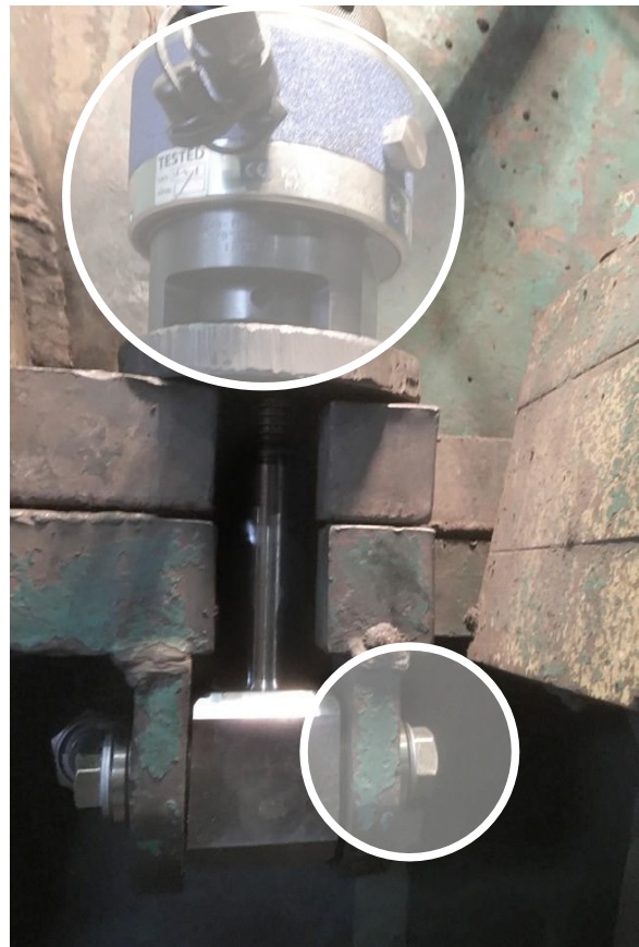
In addition to Expander (lower circle), Seinan also utilizes Boltight (top circle) from Nord Lock Group.
