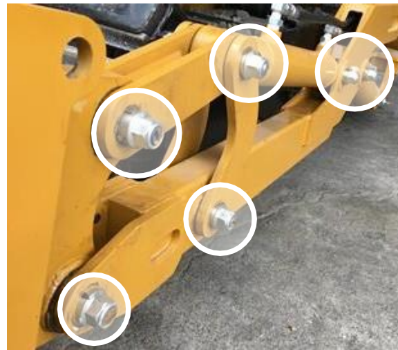
Expander is used at pivot positions to ensure minimized maintenance.
