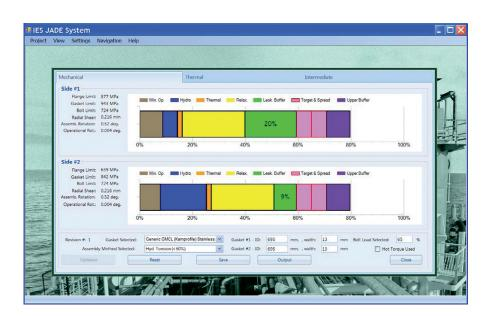
**Assembly Bolt Load Selection Graph:** these graphs allow visualization of the joint component strengths, operating loads and assembly bolt load selection. They also allow comparison of different gasket styles and dimensions. Real-time assessment means that it is possible to determine the optimal joint configuration or the reason for existing joint leakage in only a few clicks.
