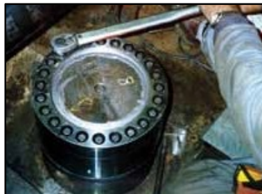
Armored Torquenut® on large machinery. Recessed jackbolts can be helpful when there is flying debris or when more thread engagement is needed.
