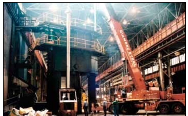
The worlds largest Torquebolt® being installed on a large hydraulic forging press.
