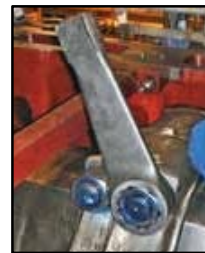
Original nuts were replaced with Superbolt® Torquenuts® on this connecting rod. Accurate preload was achieved quickly with a 3/8" torquewrench, increasing worker safety.
