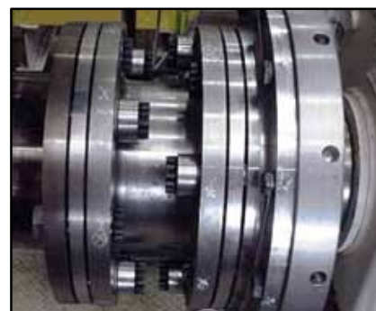
This flexible disc coupling took 2 men 2-1/2 hours to install, saving this company 19 man hours!
