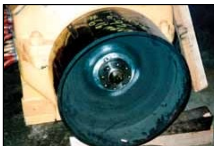
Mill Motor Nuts - SMX Series on crane motor brake drums.
