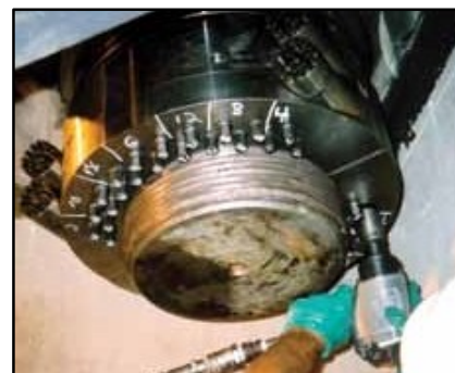
16-1/2" split nut on forging press columns.
