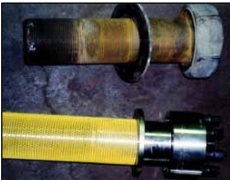
Original bolt (top) and replacement Torquebolt (bottom).
