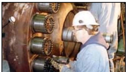
Two workers needed only 1 hour and 21 minutes to tighten these 5" tensioners.
