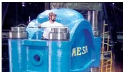
8 Superbolt® column nuts required only 12 man hours vs. 2-1/2 full days for heating of columns.
