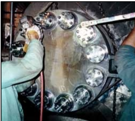
Torquebolts are also available for high temperature service and can be made from a variety of materials. Includes external installation hex on bolt heads for ease of use.
