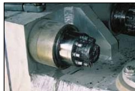
EAF Electrode Arm Assembly.
