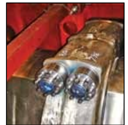
Original nuts were replaced with Superbolt® Torquenuts® on this connecting rod. Accurate preload was achieved quickly with a 3/8" torquewrench, increasing worker safety.
