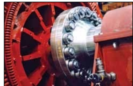
SJX-250-4 on electric motor coupling.
